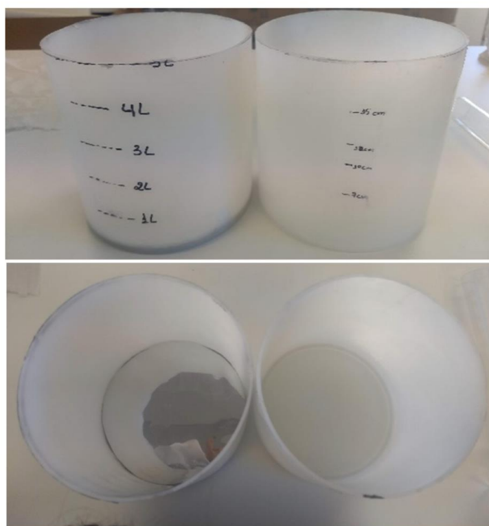
FIGURE II.3.13 – Lab-scale reaction vessels used for experiments, with and without a reflective surface
