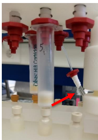
FIGURE II.3.5 – Evaporation under nitrogen flux
