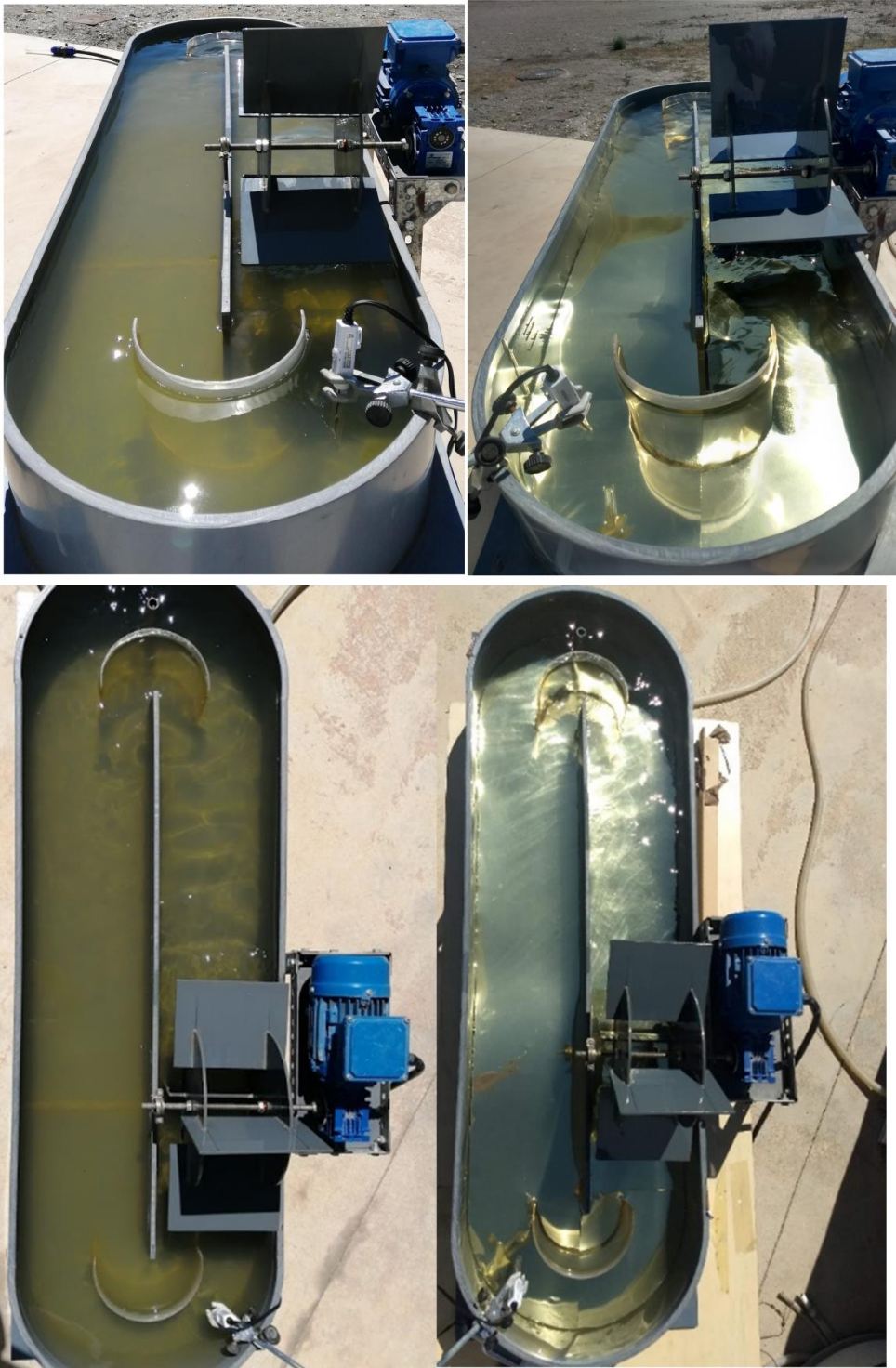
FIGURE II.3.16 – Raceway pond reactors, with and without the aluminum surface on the bottom.
