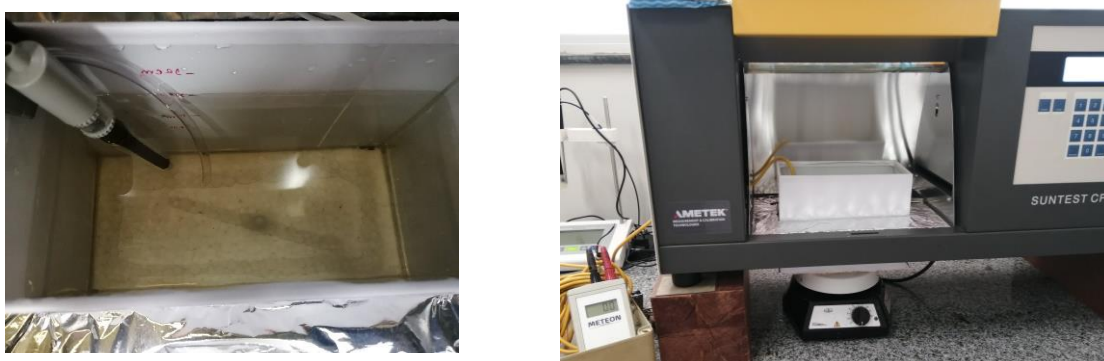
FIGURE III.3.4 – Glass covered reactor in the inside and as positioned in the SunTest CPS+ (ATLAS)
