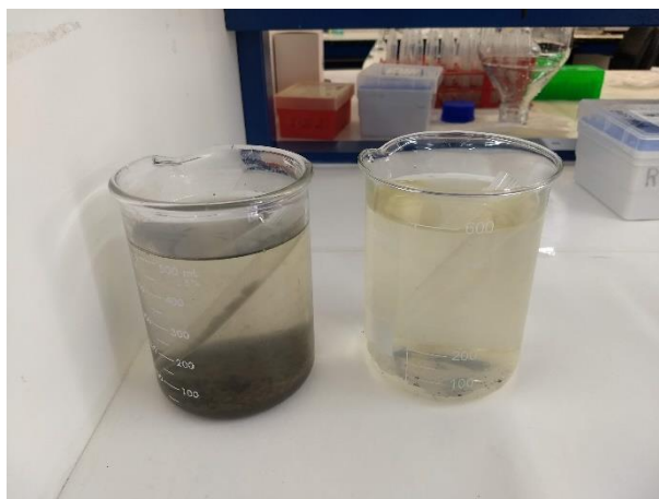
FIGURE II.3.12 – Secondary effluent from MWWTP El Ejido aspect before and after filtration
