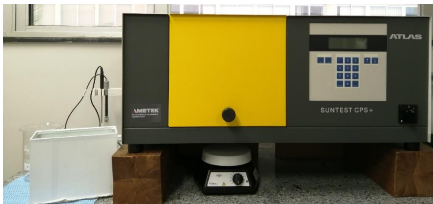
FIGURE III.3.3 – SunTest CPS+ (ATLAS) and covered glass reactor (right side)
